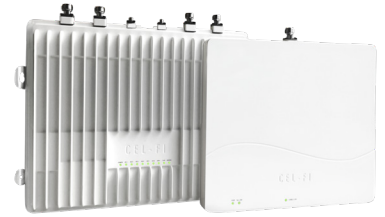
Network Unit (NU) Coverage Unit (CU)
